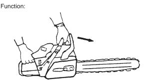
• When the lever is pushed forward, chain brake instantly works to stop the chain.
